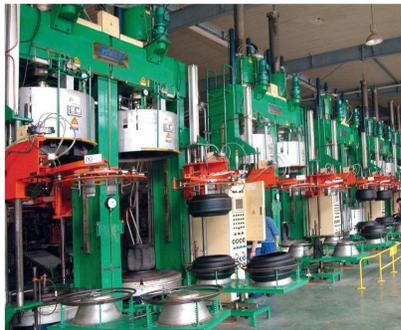
6. Steel-belted radial tire hydraulic dual-mould curing press
