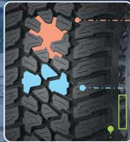
The coupled design of irregular pattern block provided enhanced traction/grasp performance.
