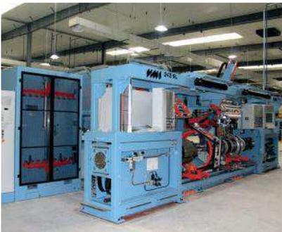
5. Single stage tire building machine of HOLLAND VMI
