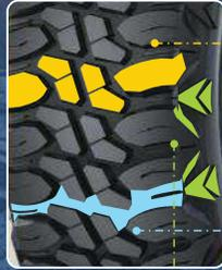
The deep shoulder pattern design and wide pattern block provide extreme grip force, which ensured the excellent handling and safety performance for the vehicle on the severe condition such as mountain and muddy road etc.
