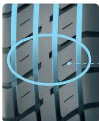
Optimized block pattern and skid proof transverse groove design endows tire stronger grip ability on dry and wet roads and more flexible and stable operation.
