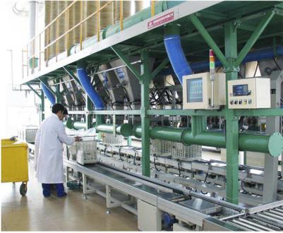
1. Automatic chemical powder weighing system for mixer
