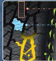
Rectangle shoulder and wide tread design with 3D multiple thin sipes increases road contact area, provides superior handling on both wet and dry surfaces, and enhances wear-resisting performance.
