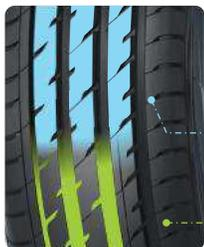
Outside strong blocks design enables the tyre to follow the road's surface contours more closely, helps to reduce blocks deformation while speed cornering, and enhances steering precision & better grip.
